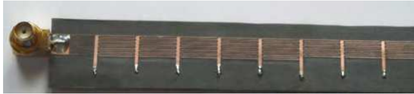
Fig. 43. A prototype and its detail of Radiation patter of tapered 16 unit-cell CRLH-TL LWA made on Rogers RT/duroid 5880.
