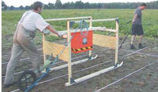
Fig. 12. Experimental setup to determine the coefficient of reflection. A 1-GHz horn antenna is mounted on a sledge 0.5 m above the ground.
