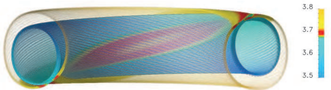
Fig. 14. A single magnetic field line showing two reconnecting flux surfaces. Its color is proportional to the local \lambda value (the color scale is indicated on right). The outer surface has a higher \lambda than the inner surface. The helical reconnection layer adopts an intermediate value.
