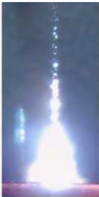
Fig. 2. Photography of ns laser ablation from Nd:YAG laser in air atmosphere. Ablation of material leads to ejection of cluster particles that may be irradiated by subsequent laser pulses.
