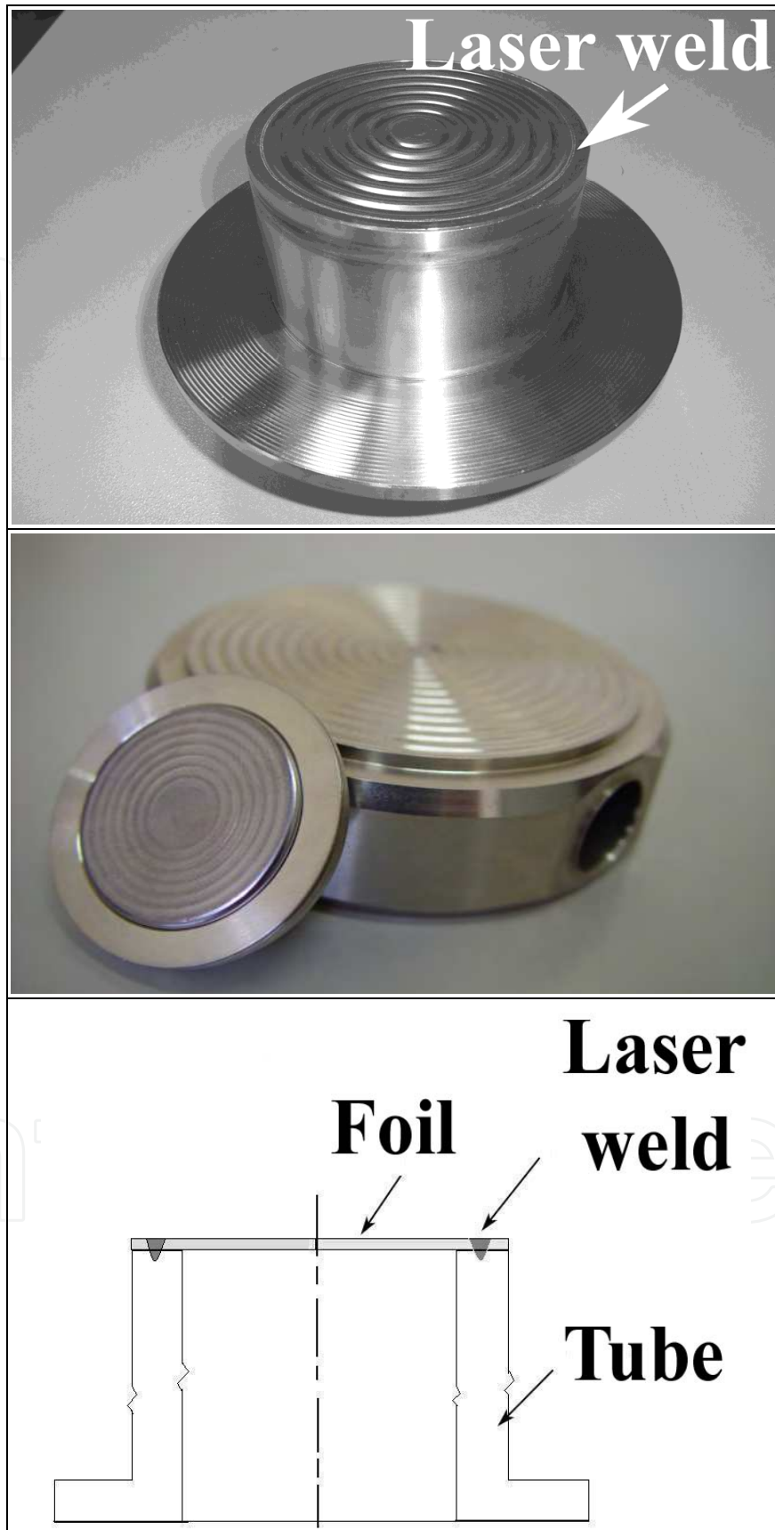
Fig. 1. Chemical seal welded by pulsed Nd:YAG laser.
