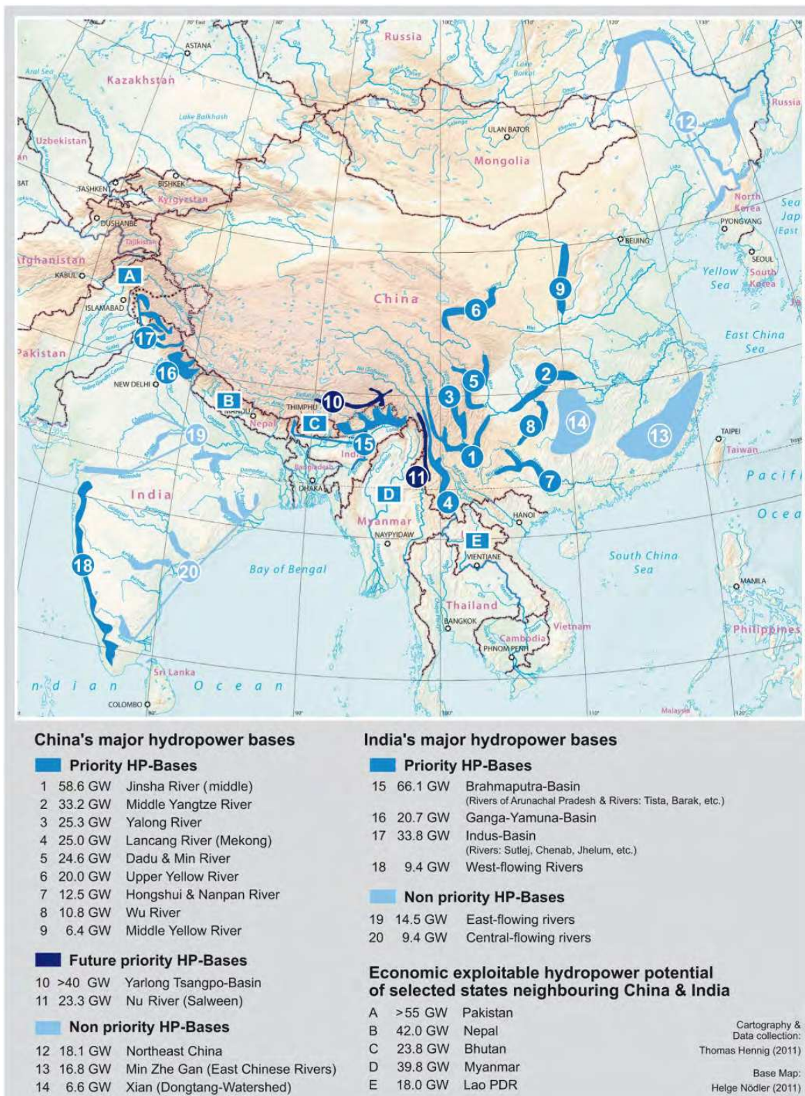
Fig. 3. Economic exploitable hydropower potential of China's and India's hydropower bases as well as of selected neighbouring states.
