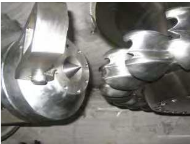
Photo 37. A deflector before the commissioning (case study le Châble Profray).
