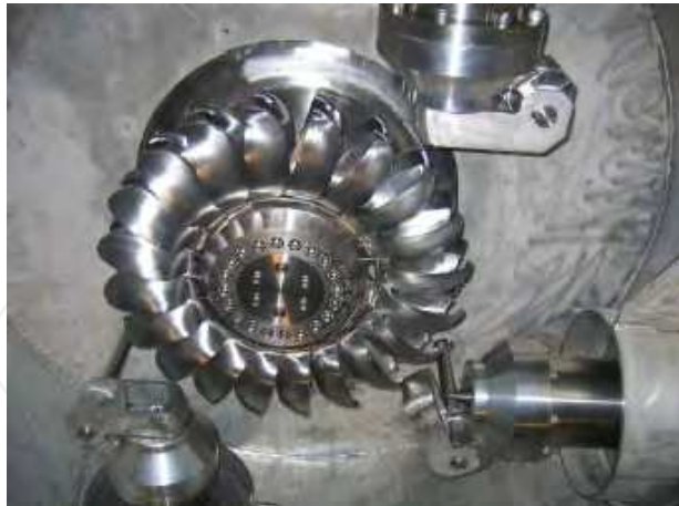
Photo 29. The Pelton runner and its 3 jets (case study La Zour).
