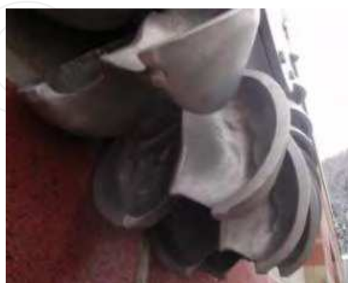
Photo 32. Pelton bucket worn out by sand particles (case study Le Châble-Profray).
