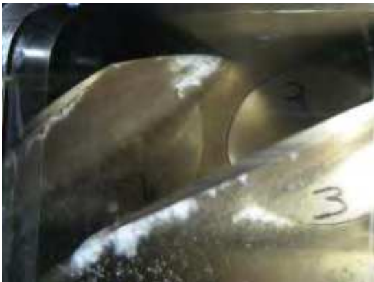
Photo 35. Cavitation on blades for a Kaplan runner.
