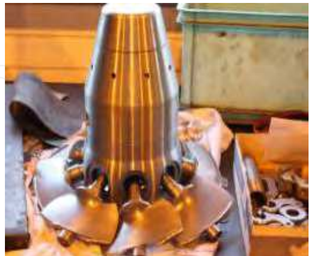
Photo 28. Kaplan runner with 8 blades during manufacturing, to be set within a drinking-water network (case study Poggio Cuculo).
