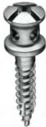
Fig. 7. The screw used in the proposed case has the following features: 2.0mm screws, 8-12mm thread lengths, made of 316L extra-hard stainless steel for maximum strength; self-drilling, self-tapping for one-step insertion; groove under screw-head secures wires or elastics; cruciform head design; two cross-holes with align cruciform head slots; a 4-mm capstan-style head to hold the wire away from the mucosa (Synthes, West Chester, Pennsylvania).
