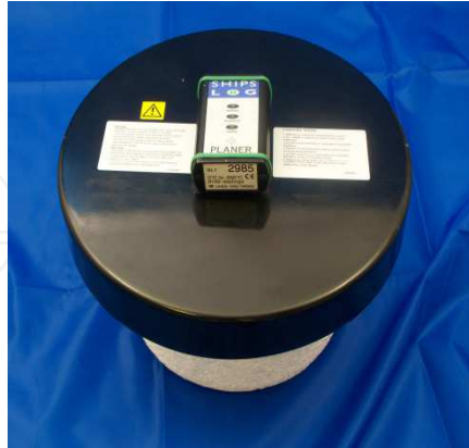
ShipsLog datalogger for vapour shippers
