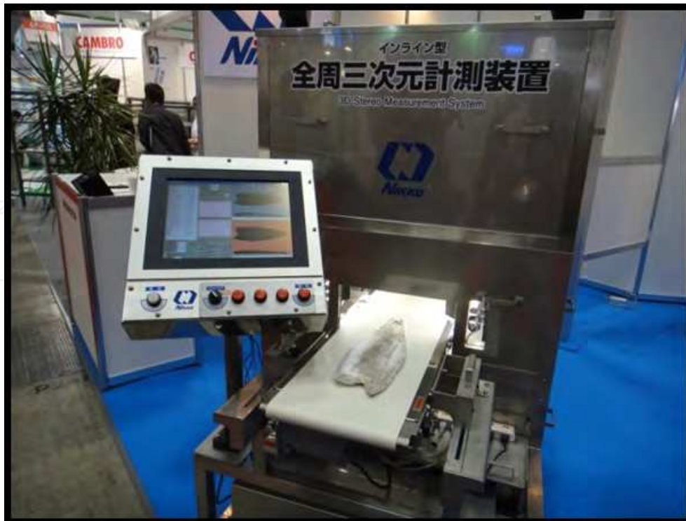
Fig. 11. 3D measurement system that it developed jointly with the National Institute of Advanced Industrial Science and Technology (Anonymous, 2011a.).
