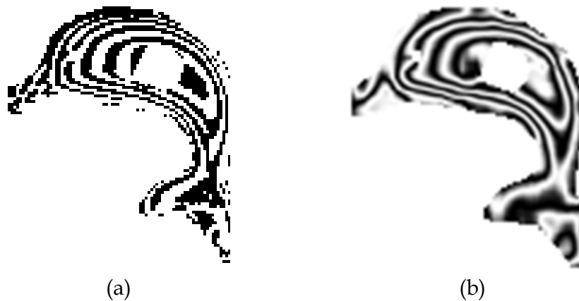
Fig. 15. (a) Result of binarize fig 14; (b) Fringe pattern associated with the demodulated phase.
