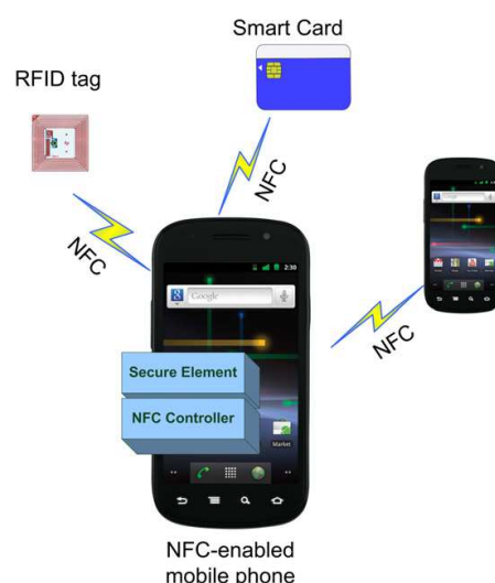
Fig. 4. NFC-enabled phone operating modes.
