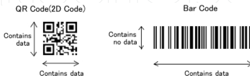
Fig. 2. QR Code compared with a Bar Code [Source: http://www.qrcode.com/aboutqr-e.html ]
