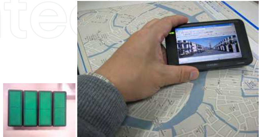
Fig. 3. Digital scope by a lightweight high-resolution display receiving data signal through the 2D sheet. The connector for the display contacts the sheet to receive the power signal.
