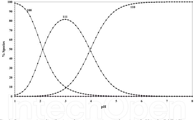
Fig. 3. Concentration distribution of various species as a function of pH in the Pd(DAP)-Glutathione system at concentrations of  $1.25 \times 10^{-3}$  mol-dm<sup>-3</sup> for Pd(DAP)<sup>2+</sup> and glutathione, I = 0.1 mol-dm<sup>-3</sup> (NaNO<sub>3</sub>) and T =  $25 \pm 0.1$  °C).
