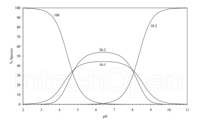
Fig. 1. Concentration distribution of various species as a function of pH in the  $Pd(AMBI)(H_2O)_2$  system at concentration of  $1.25 \times 10^{-3}$  mol-dm<sup>-3</sup>, I = 0.1 mol-dm<sup>-3</sup> (NaNO<sub>3</sub>) and T =  $25 \pm 0.1$  °C).
