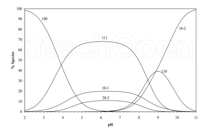
Fig. 2. Concentration distribution of various species as a function of pH in the Pd(AMBI)-Ornithine system at concentrations of  $1.25 \times 10^{-3}$  mol-dm<sup>-3</sup> for Pd(AMBI)<sup>2+</sup> and ornithine, I = 0.1 mol-dm<sup>-3</sup> (NaNO<sub>3</sub>) and T =  $25 \pm 0.1$  °C).
