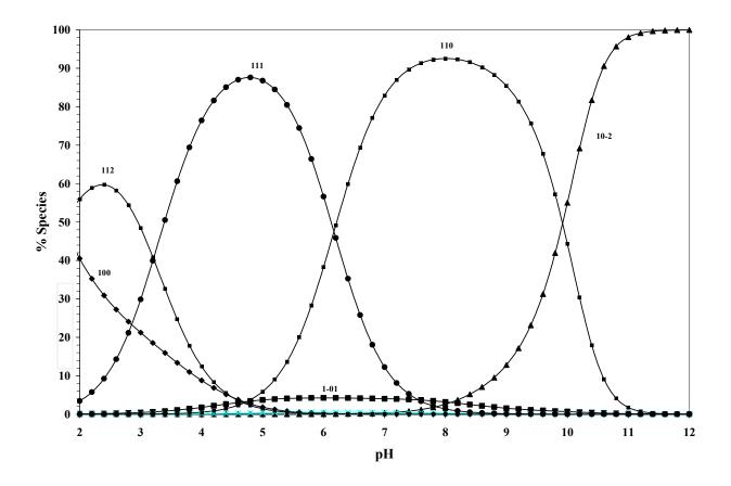
Fig. 4. Concentration distribution of various species as a function of pH in the Pd(AMBI)-5<sup>-</sup>-GMP system at concentrations of  $1.25 \times 10^{-3}$  mol-dm<sup>-3</sup> for Pd(AMBI)<sup>2+</sup> and 5<sup>-</sup>-GMP, I = 0.1 mol-dm<sup>-3</sup> (NaNO<sub>3</sub>) and T =  $25 \pm 0.1$  °C).
