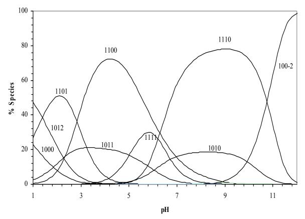
Fig. 5. Concentration distribution of various species as a function of pH in the Pd(Pic)-CBDCA-IMP system at concentrations of  $1.25 \times 10^{-3}$  mol-dm<sup>-3</sup> for Pd(Pic)<sup>2+</sup>; CBDCA and IMP, I = 0.1 mol-dm<sup>-3</sup> (NaNO<sub>3</sub>) and T =  $25 \pm 0.1$  °C).
