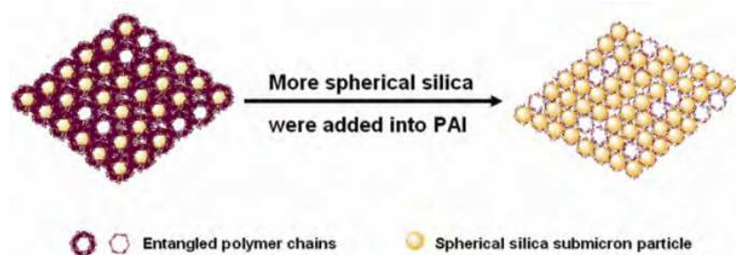
Scheme 3. Interactions between the silica submicron particles and the PAI polymer matrix.
