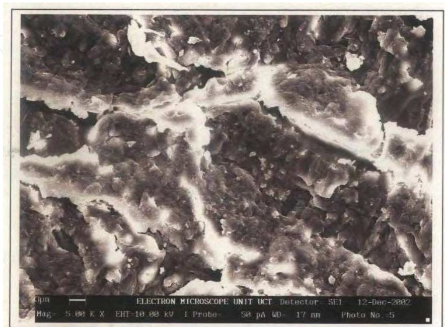
Fig. 4. Micrograph of outer surface of raw coconut shell Source: Achaw & Afrane, 2008
