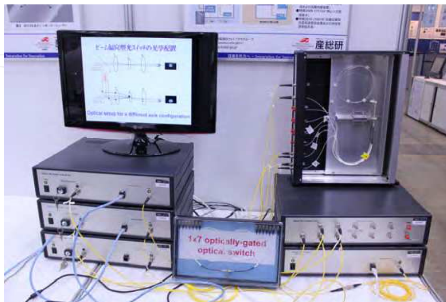
Fig. 15. External view of “The least stand-by power system using a 1x7 all-optical switch”.
