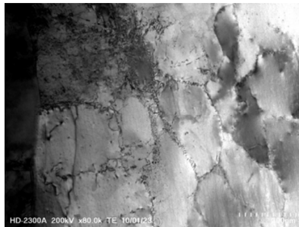
Fig. 14. Microstructure of Cu after COT deformation at: f=1,8 Hz, \alpha =6^\circ , v=0,015 mm/s and \Delta h=7 mm
