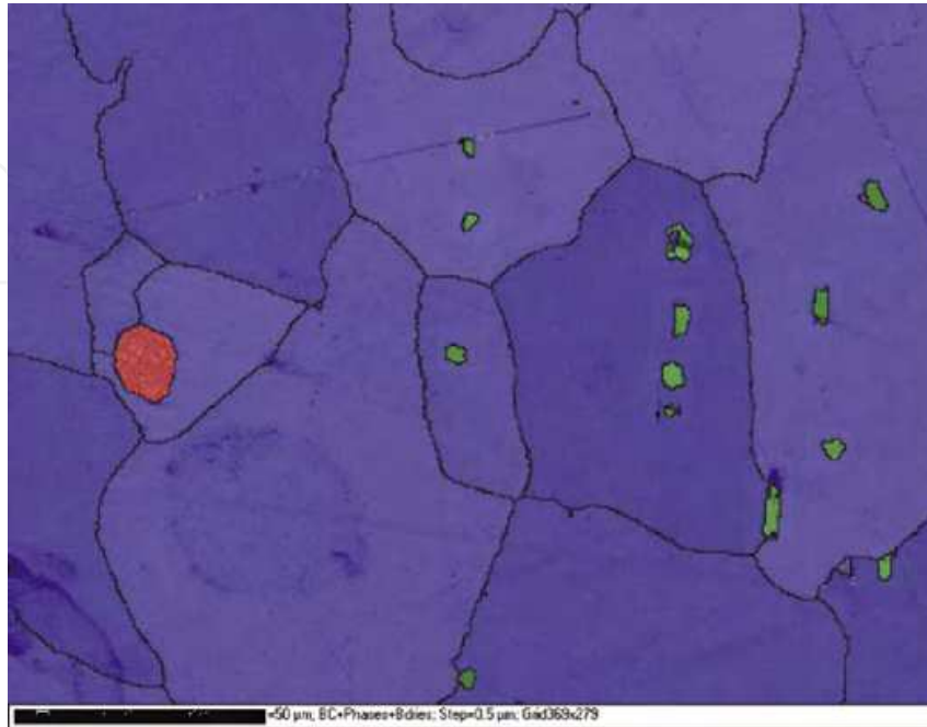
Fig. 3. Phase map showing the same area imaged in Fig. 1. Blue = ferrite, Red = AlN and Green = \text{Cr}_{23}\text{C}_6 . Black lines represent grain boundaries.
