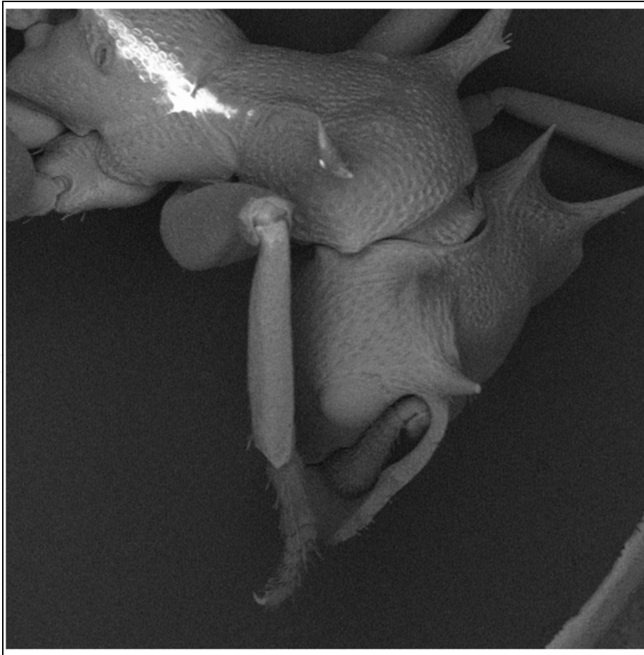
Fig. 2. SEM image of a biological sample(cephalotes) using quad backscattered detector. The sample was not sputter coated resulting in excessive charging(white area) on the sample.
