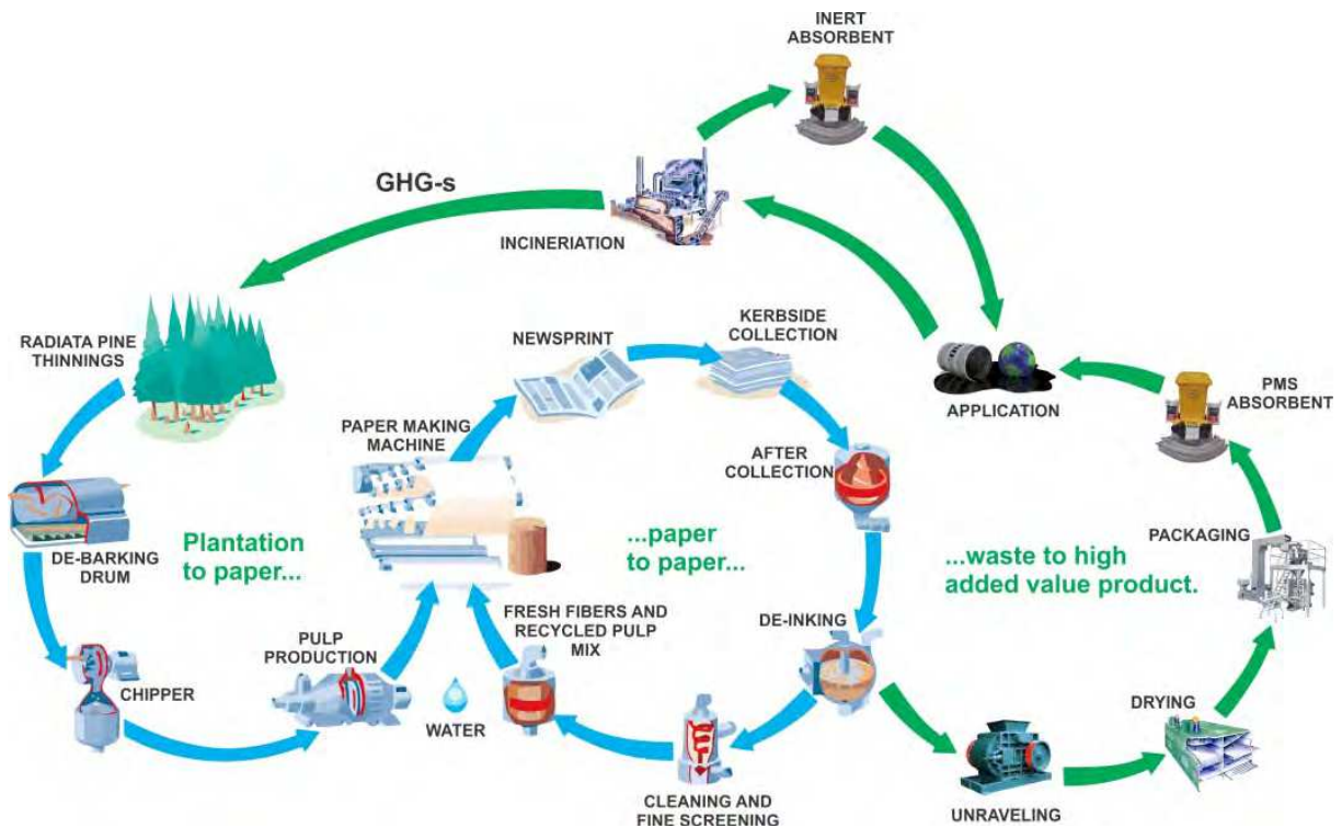
Fig. 10. Life cycle of paper in the case of conversion of PMS into sorbent material.
