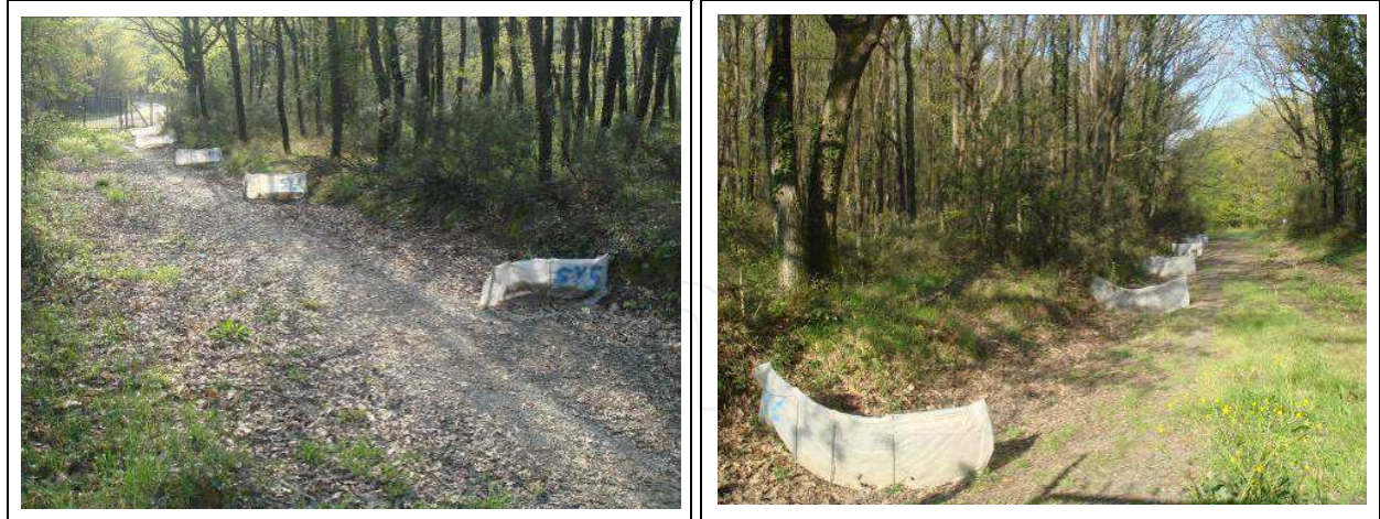
Fig. 4. Sediment traps on forest road and collected sediments on sediment traps at Belgrad Forest-Istanbul, Turkey (Kartaloğlu, 2011).
