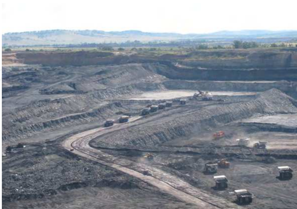
Fig. 8. A view of a truck and shovel operation in Hunter Valley Region in NSW.
