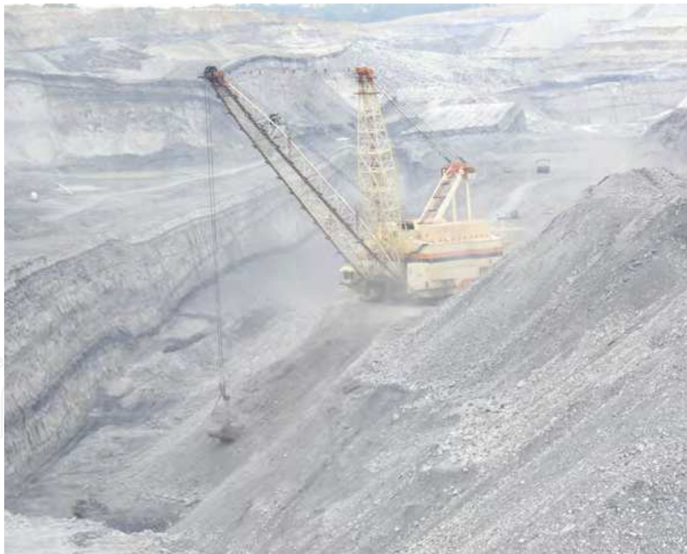
Fig. 6. A typical dragline in operation in Hunter Valley Region in NSW.
