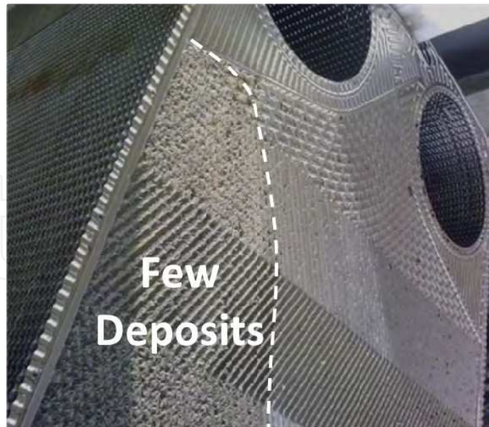
Fig. 8. Deposits formed on the surface of NT-plate.
