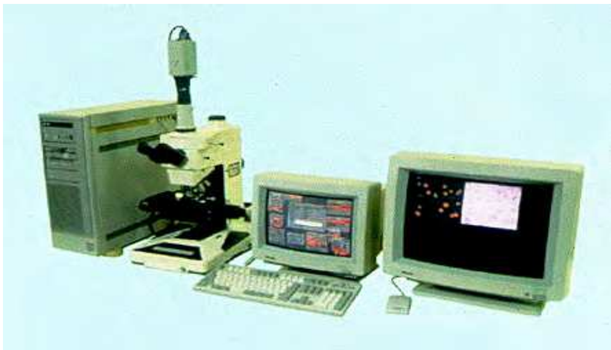
Fig. 2. IPAP system. This system is comprised of a microscope, a CCD color video camera and an analyzing computer for converting microscopic photographic images into digital images.
