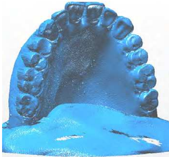
Fig. 4. The polygon mesh resulted from 3D scanning of the maxillary complete denture
