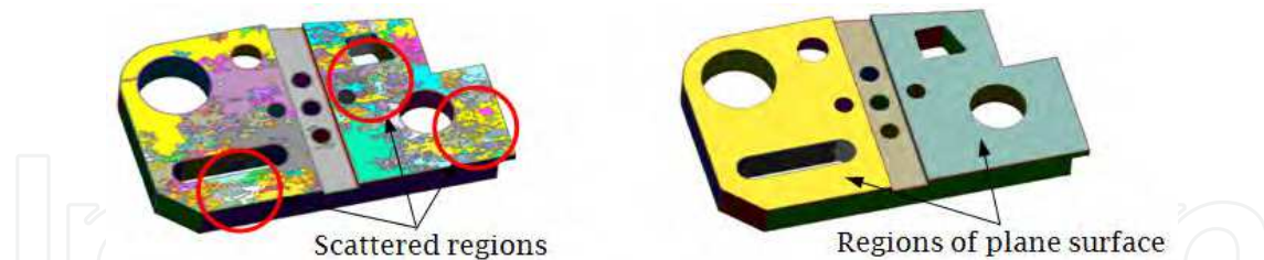
Fig. 4. Example of mesh segmentation, (a) an object segmented into many small regions due to a high sensitivity threshold, and (b) regions determined with a low sensitivity threshold
