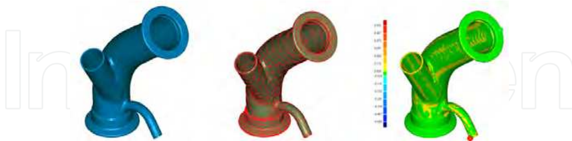
Fig. 9. Results of the tubing example tested using Geomagic , (a) polygon mesh (589,693 triangles), (b) NURB model (1,107 patches), and (c) deviation analysis
