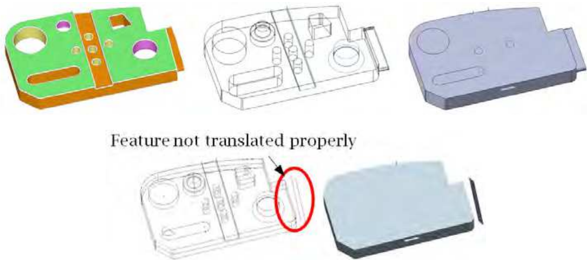
Fig. 21. The block model explored to SolidWorks and Wildfire , (a) seventeen features recognized in Geomagic , (b) features exported to SolidWorks (wireframe), (c) features "piled up" in SolidWorks , (d) features exported to Wildfire (wireframe), and (e) features "piled up" in Wildfire
