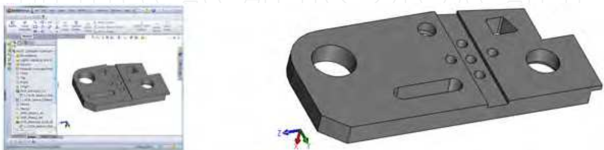
Fig. 22. Block exported from Rapidform to SolidWorks , (a) solid model exported to SolidWorks , and (b) design change made in SolidWorks
