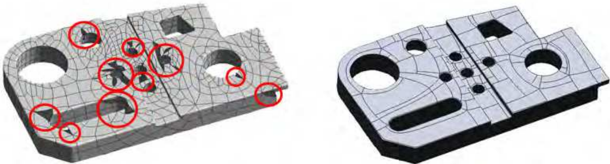
Fig. 11. NURB surface models generated using two different options in Rapidform , (a) Evenly Distribution Network option, and (b) Feature Following Network option
