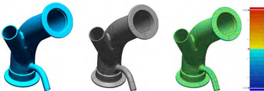
Fig. 14. Results of the tubing example tested using Rapidform , (a) polygon mesh (589,693 triangles), (b) NURB surface model (185 patches), and (c) deviation analysis
