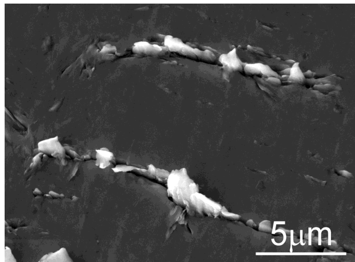
Fig. 30. Cyclic slip bands on the surface of UFG Cu loaded in HCF region
