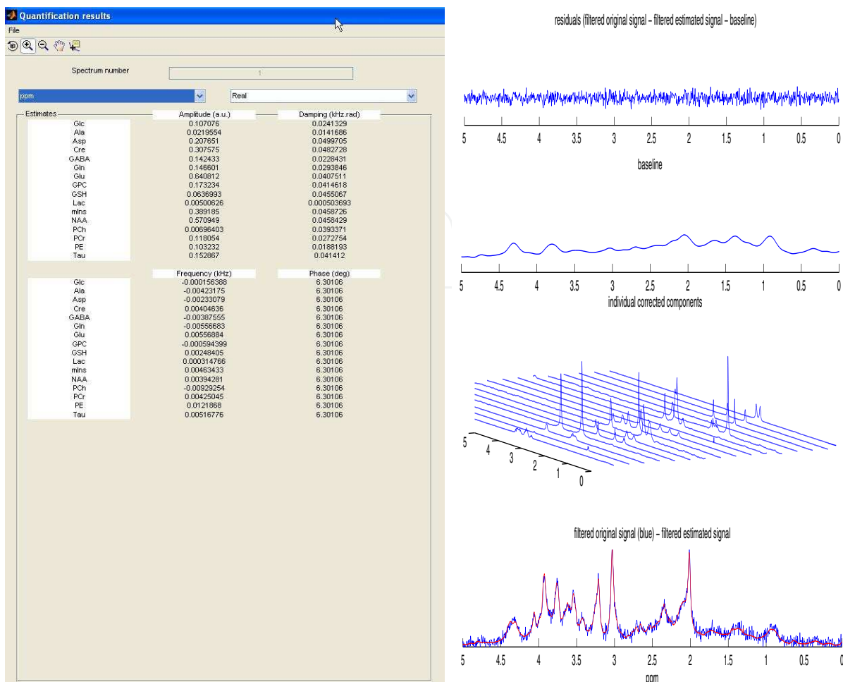
Fig. 2. Quantification results window for AQSES in SPID (left side) of an in vivo 1 H MRS signal from mouse brain acquired with a 9.4 T Bruker Biospec small animal MR scanner (Bruker BioSpin MRI, Ettlingen, Germany) with acquisition parameters: PRESS sequence, TR=4 s, TE=12 ms, SW=4 KHz, NDP=2048 points and 256 averages, volume of interest (VOI)= 3 × 1.75 × 1.75 mm 3 . The basis set of 16 metabolites used for quantification was measured in vitro . Right: plots of residue, splines baseline, estimated metabolites and original with estimated signal.
