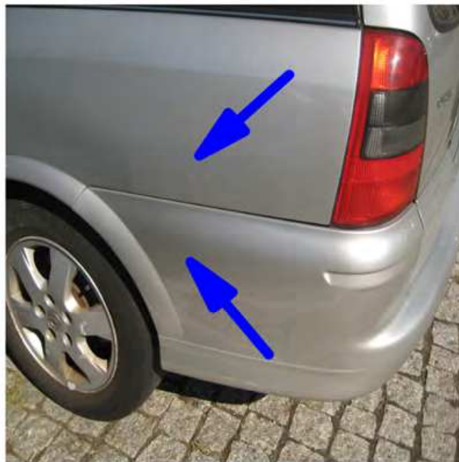
Fig. 3. Example of colour harmony in a silver-like coating containing aluminium flakes. Current colour designs must achieve no perceptible colour differences between the different external parts that integrate the car such as the car body and the fenders.
