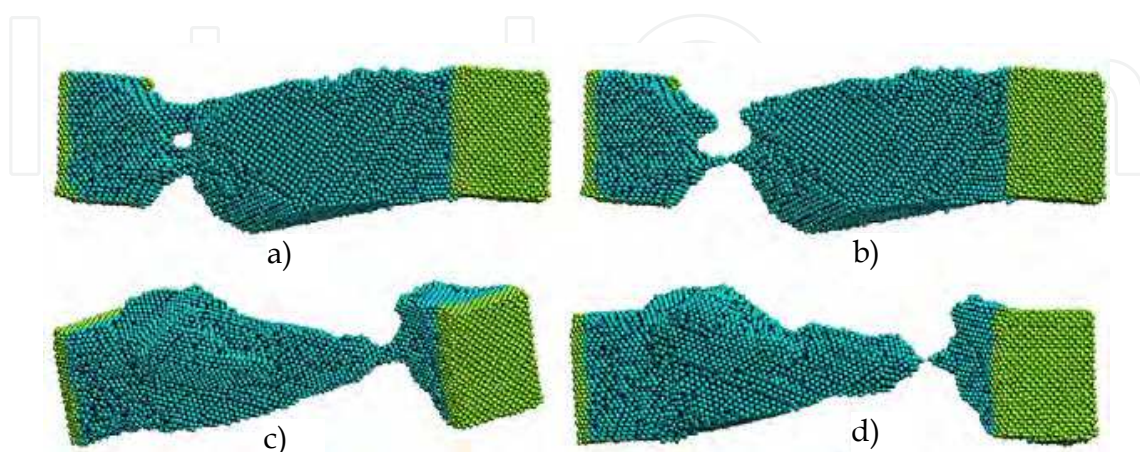
Fig. 18. (a) and (b) the formation of rupture of specimen with no defects for shear simulation, (c) and (d) that of specimen with scratching depths of 5a_0 .
