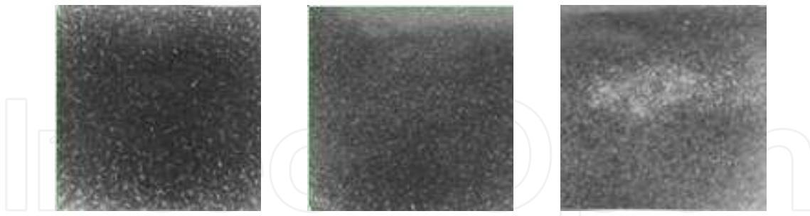
Fig. 19. Defect texture, from left to right: shrinkages of needle cavity and small round cavity as well as sponge shrinkage
