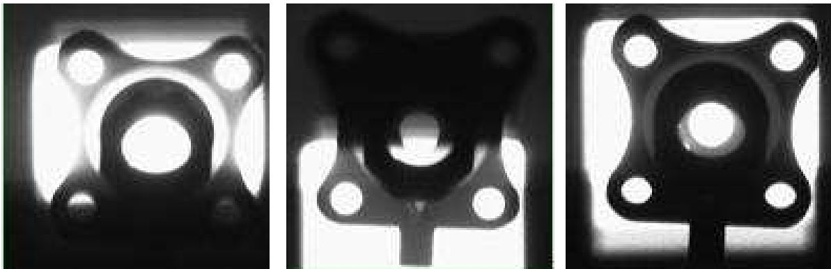
Fig. 11. The radiographs with different tube voltage for the same specimen, the tube voltage used from left to right are separately 110KV, 105KV and 75KV and all with tube current 1.5mA
