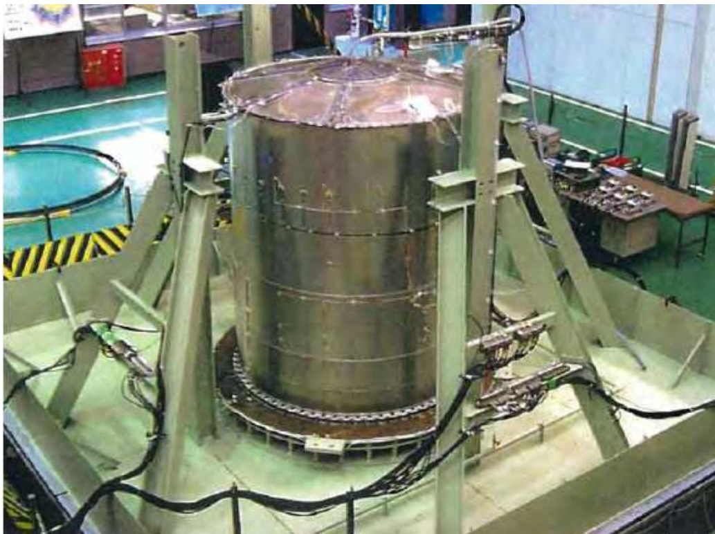
Fig. 19. Large test tank of 1/5 reduced-scale cylindrical liquid storage tank. (Ito et al., 2003)
