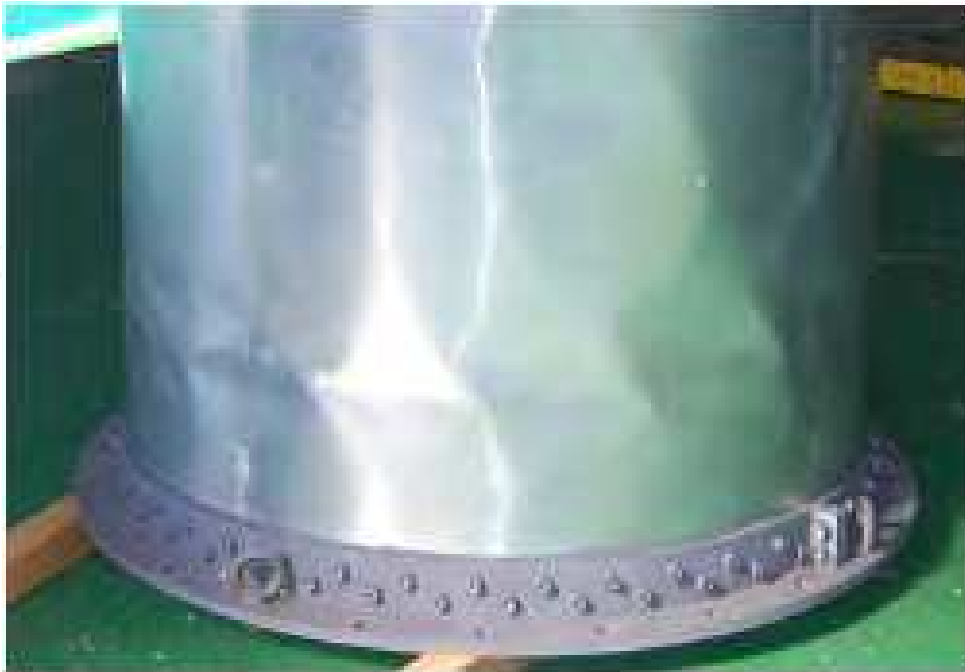
Fig. 2. Typical mode of diamond buckling.
