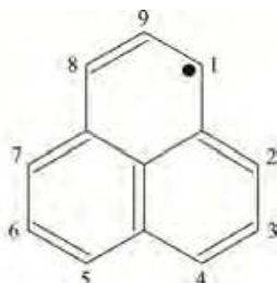
Fig. 18. Structural representation to perinaphthenyl radical indicating, 1 to 9, hydrogen atoms responsible for the hyperfine splitting observed in marine diesel spectrum.
