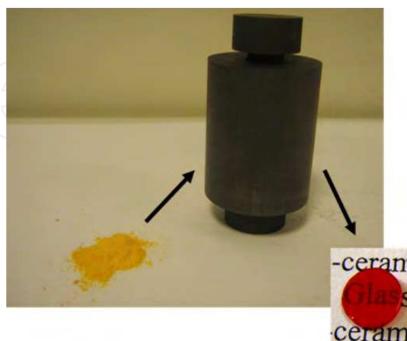
Fig. 10. Photograph of the processed glass sample for the composition 62.5\text{GeS}_2\text{-}12.5\text{Sb}_2\text{S}_3\text{-}25\text{CsCl} .
