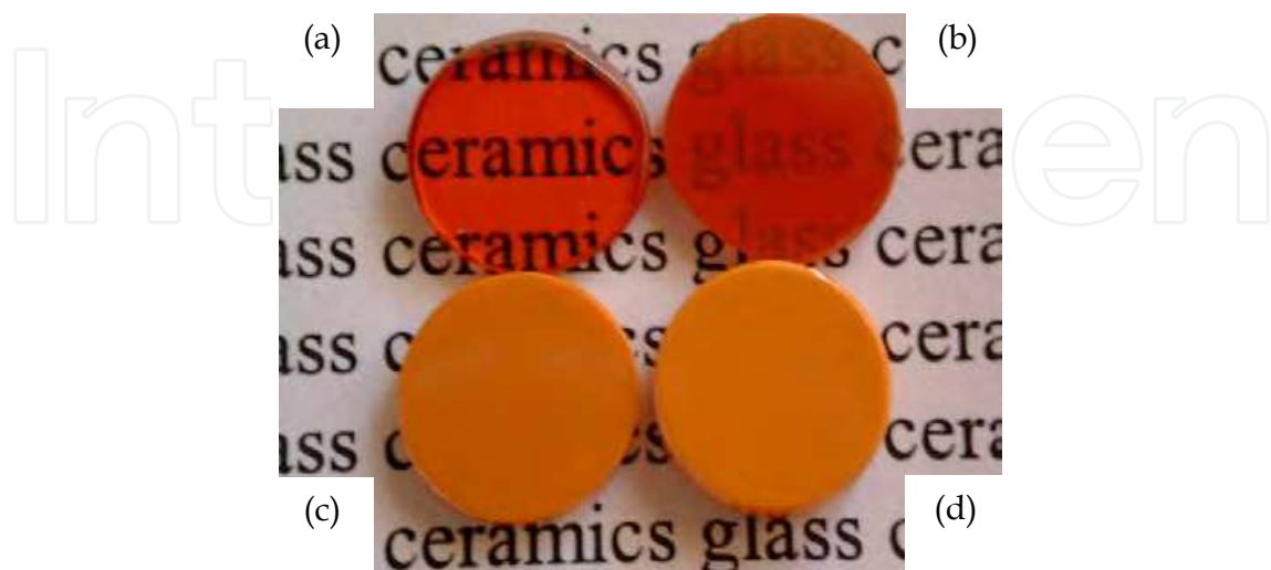
Fig. 5. Glass composition 62.5\text{GeS}_2\text{-}12.5\text{Sb}_2\text{S}_3\text{-}25\text{CsCl} heated at 290^\circ\text{C} for different crystallization times (a) No thermal treatment (b) 7h (c) 73h and (d) 144h.
