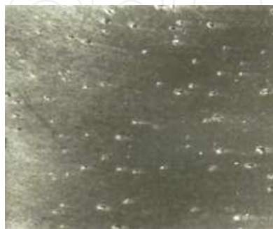
c. intensive porosity over the volume, higher pattern density and thicker coating layers, EPC process
