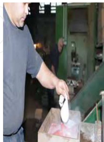
d. coating application by rag
