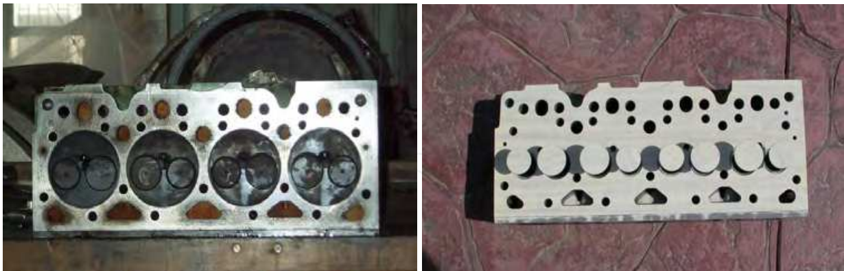
a) Cylinder heads and valves without coating b) Ceramic coated cylinder heads and valves Fig. 11. Cylinder head and valves before coating and after coating
