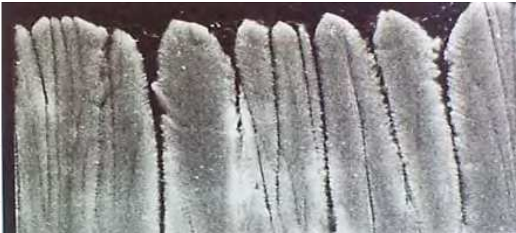
Fig. 29. The top part of a columnar coating
