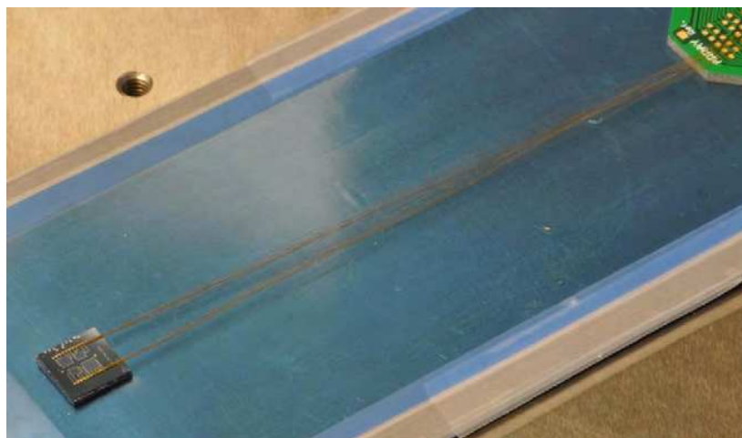
Fig. 6. Photograph of top side of a solid diaphragm sensor assembly with hydrogel inserted and mounted to a perforated backing plate (out of view). Wire bonding was performed using gold insulated wire ( d=50\ \mu\text{m} ). Reprinted from (Orthner et al., 2010b)
