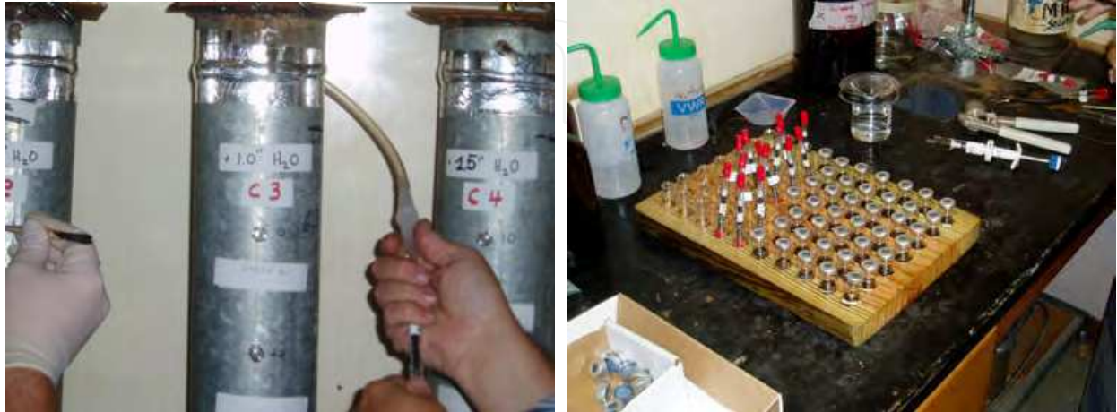
Fig. 2a. Charcoal filters replaced periodically. Fig. 2b. Charcoal filter extracted into vials.
