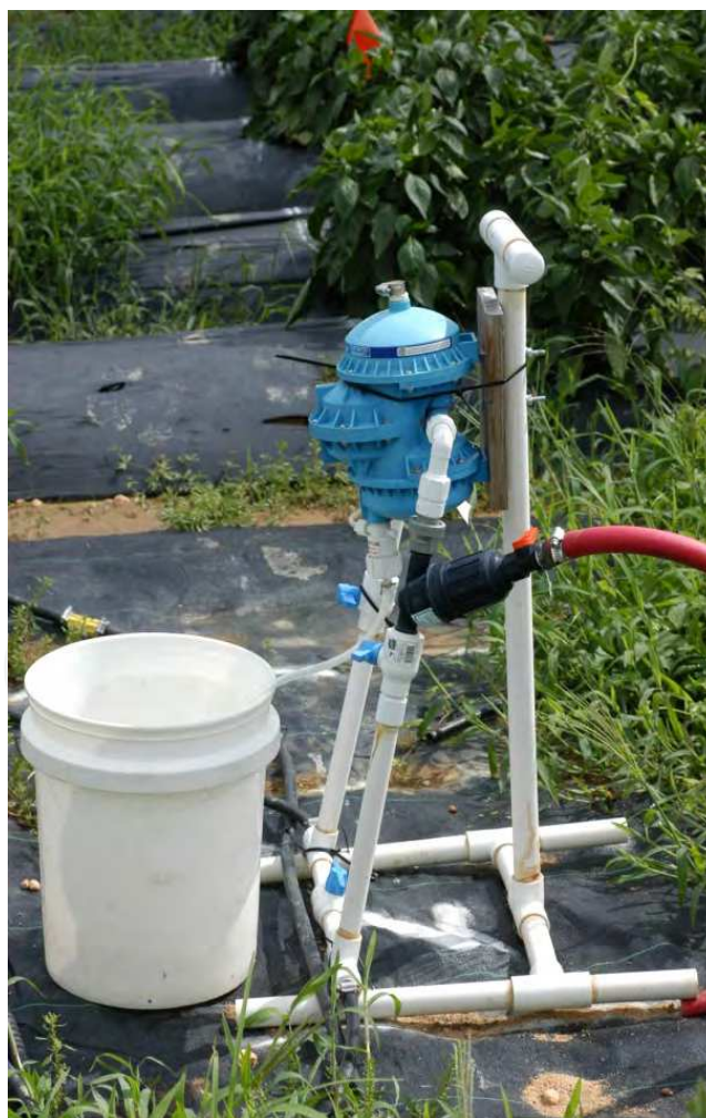
Fig. 4. A Chemilizer ® volumetric injection pump.
