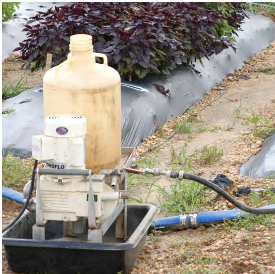
Fig. 7. A positive displacement electric (1/3 hp) metering pump with a 5-gallon jug for the concentrated insecticide solution and a containment tray beneath to catch all drips, spillage, etc. In the center of the picture is a flush valve to quickly and completely rinse all solution from within the pump.
