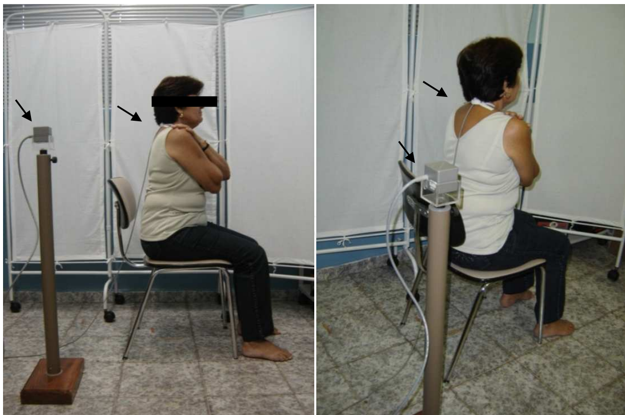
Fig. 2. Illustration of initial position for the sit-to-stand test. Arrows indicate the positions of sensor coil on the seventh cervical vertebra and the transmitting coil.
