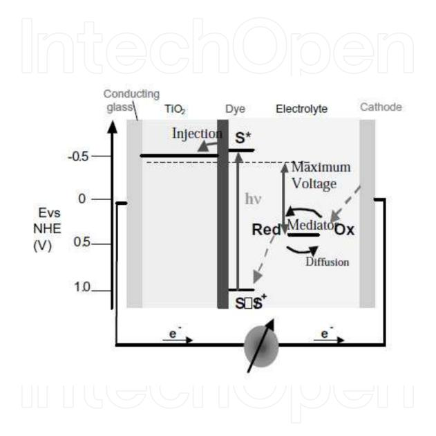
Fig. 2. A schematic presentation of the operating principles of the dye-sensitized solar cell (The figure was reproduced from Grätzel, 2003).
