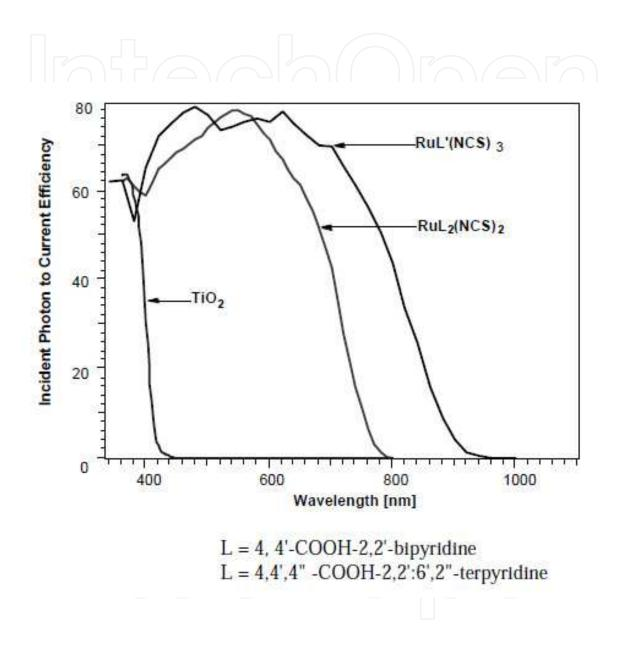
Fig. 3. The incident photon to current conversion efficiency of the dye-sensitized solar cell is plotted as a function of excitation wavelength. (The figure was reproduced from (Grätzel, 2003)).
