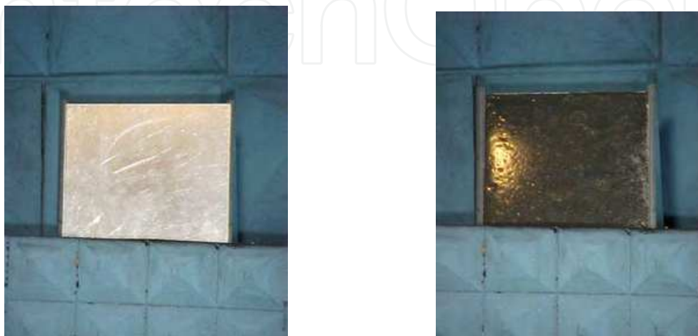
Fig. 11. Flat plate assembled in an anechoic chamber: metal face (left) and ERAM face (right).
