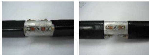
Fig. 35. The rotational shaft equipped with two SAWRs.
