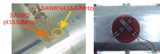
Fig. 30. The setup of the SAWRs and the strain gage on the shaft.
