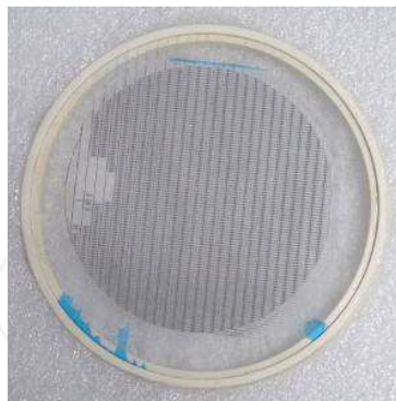
Fig. 26. The Wafer of f -tech SAWRs (433.92MHz).
