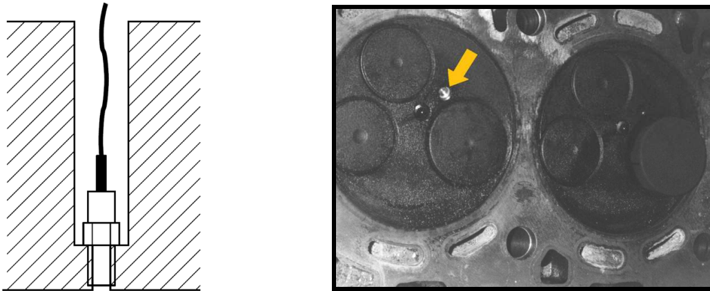
Fig. 3. Pressure transducer mounting location.
