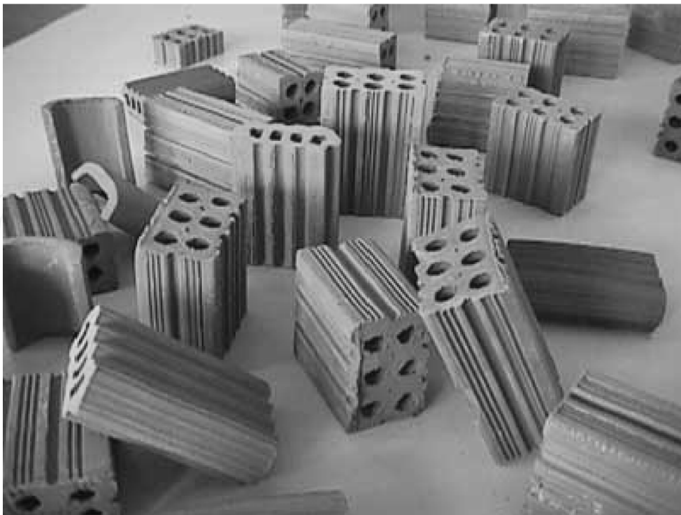
Fig. 4. Ceramic bodies containing granite sawing waste
