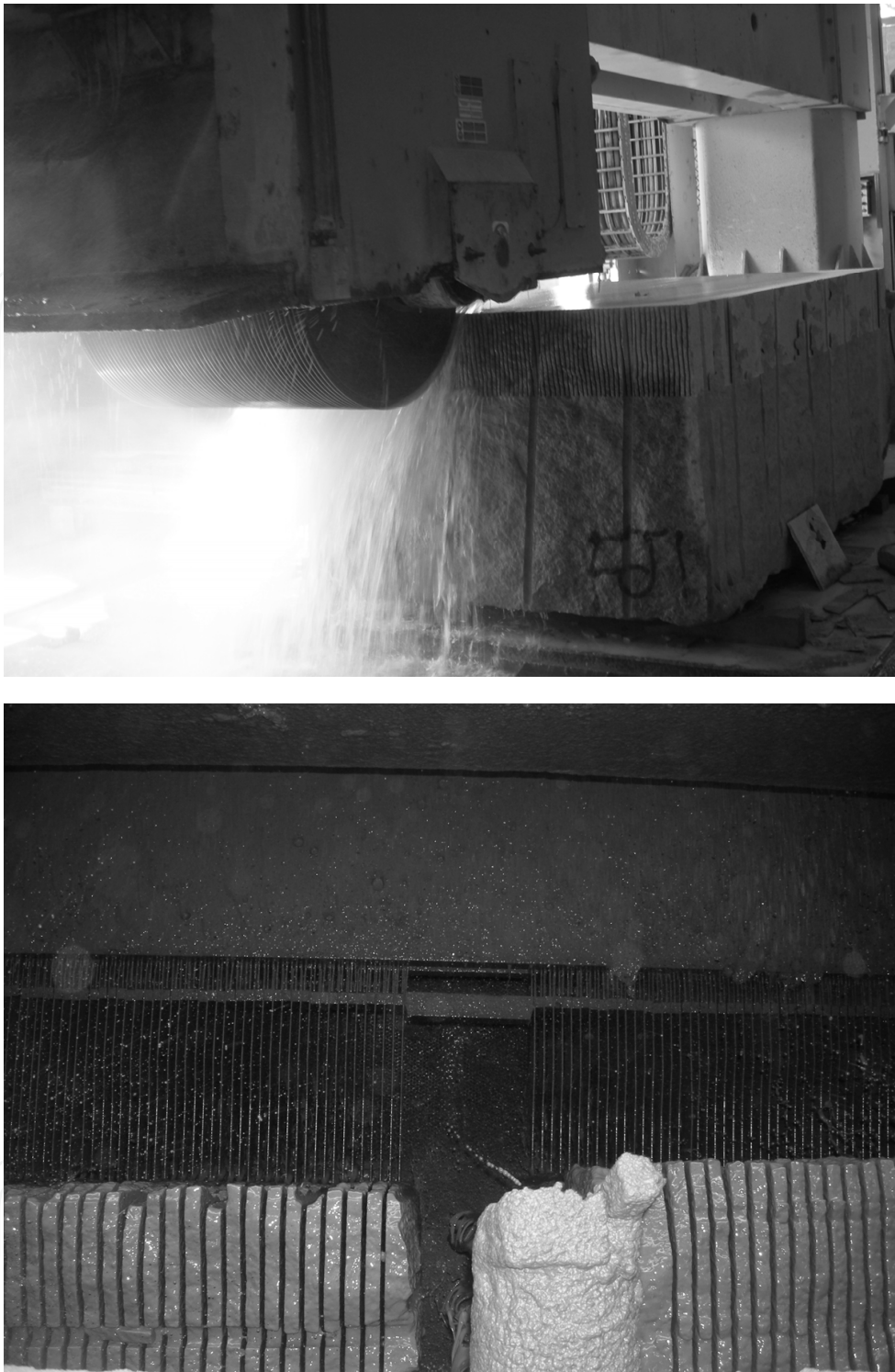
Fig. 1. Sawing operation of granite blocks.
