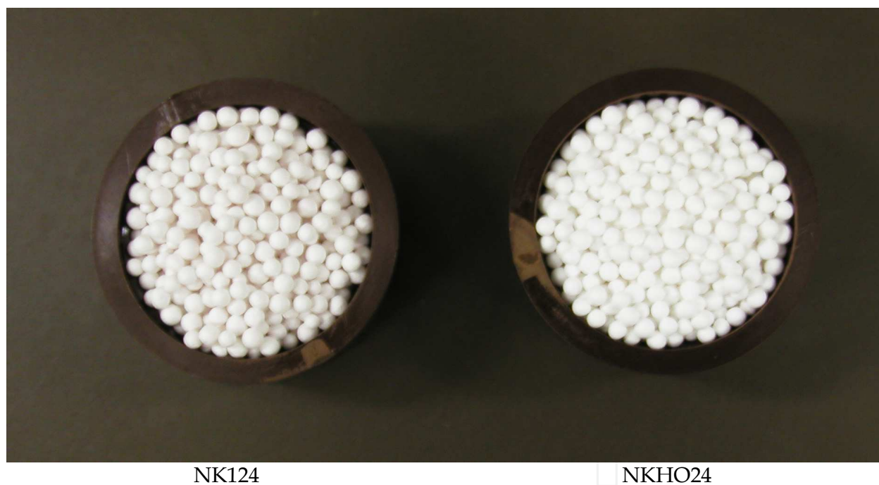
Fig. 2. Prepared alumina carrier-TiO 2 photocatalysts
