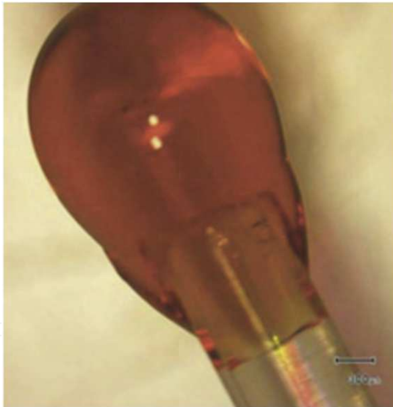
Fig. 2. Picture of the sensing probe: polymer-silica sol-gel hybrid deposited onto the tip of the POF.
