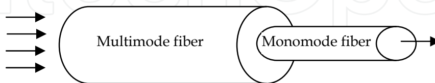
Fig. 13. Spatial mode filtering using welded multimode and monomode fibers
